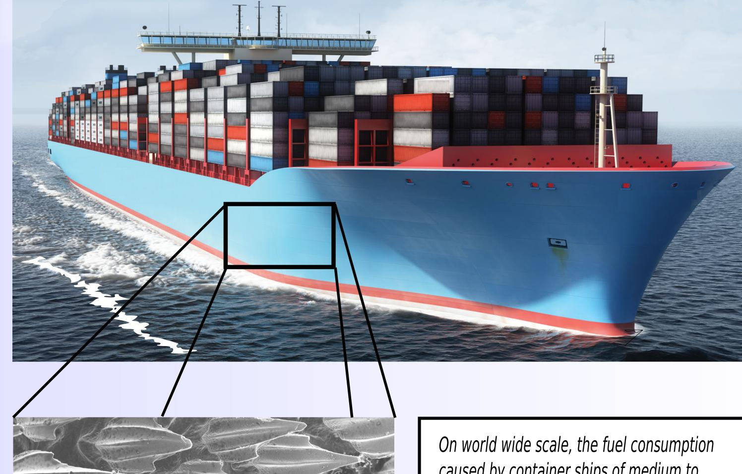
On world wide scale, the fuel consumption caused by container ships of medium to large size is about 150-250 tons per day. If shark skin like surfaces could be implemented properly on ships, a 24.6 % drag reduction would save up to roughly 16 billion kr per year and 600'000 tons of CO2 per year on container shipping alone\*\*
